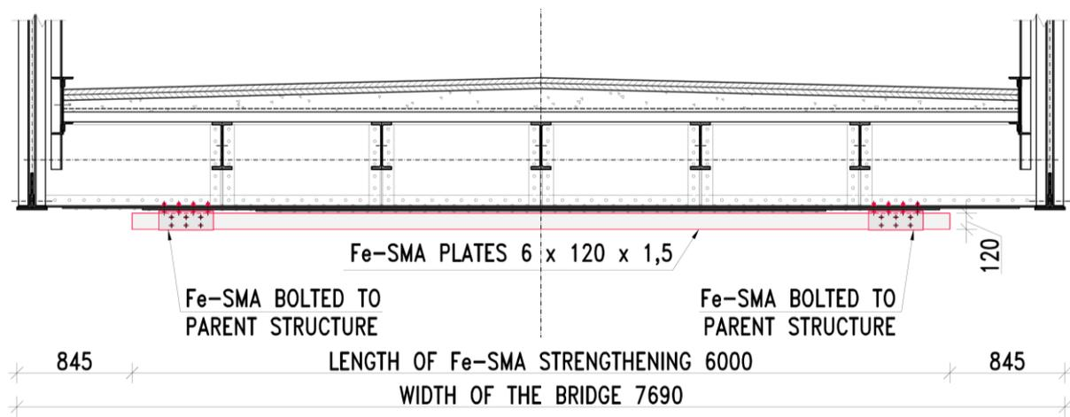
Figure 3. Cross-section of Petrov bridge deck with Fe-SMA strengthening
