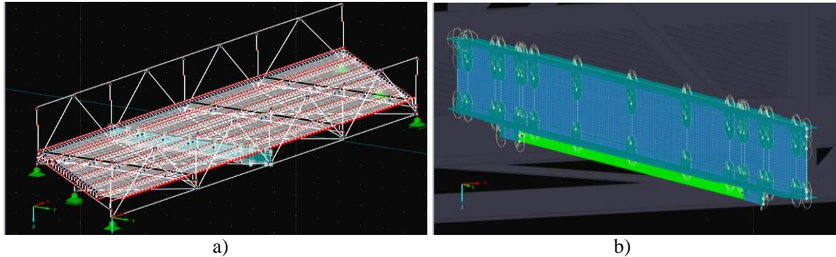
Figure 4. Numerical model: a) whole Petrov bridge b) Strengthened cross girder using shell elements.
