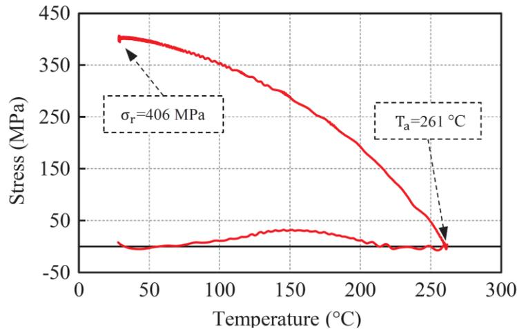
Figure 2. Stress-Temperature of Empa's Fe-SMA, Izadi et al. (2018b)
