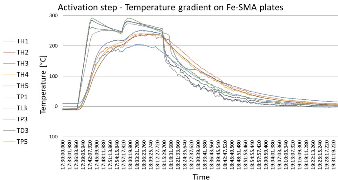
Figure 6. Typical temperature-history on the Fe-SMA plates during activation process.
