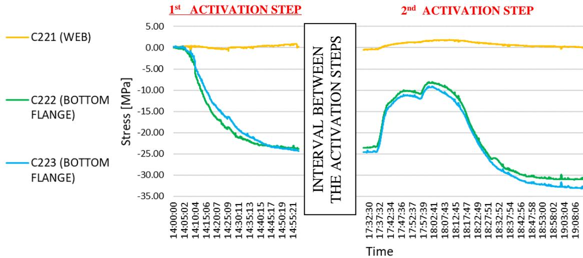
Figure. 7 Stress state of the mid-span section of strengthened cross girder during both activation steps.
