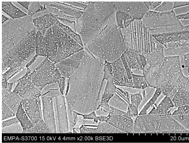
Fig. 2. SEM-BSE image of the as-received Fe-SMA.
