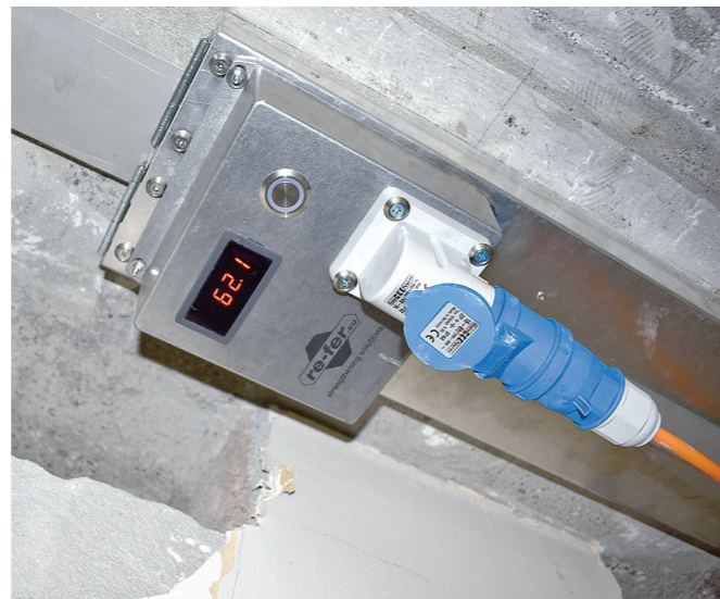
6 Program temperature control during heating via the built-in control unit log
