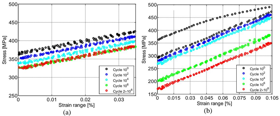
Fig. 3. SMA (activated) stress-strain behavior under fatigue loading for (a) Specimen F2 with  $\Delta\varepsilon_0 = 0.035\%$ , (b) Specimen F3 with  $\Delta\varepsilon_0 = 0.105\%$ .
