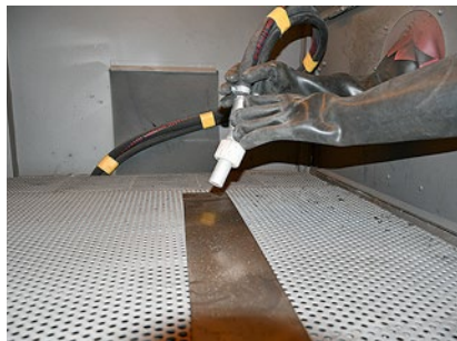
Factory sandblasting with corundum
