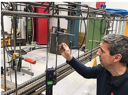
Fixing the strain gauge on internal stirrup reinforcement
