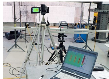
Thermal image recording of the activated/heated re-bar stirrups
