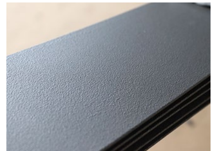
Corrosion protection with SikaCor® EG-1 applied in factory
