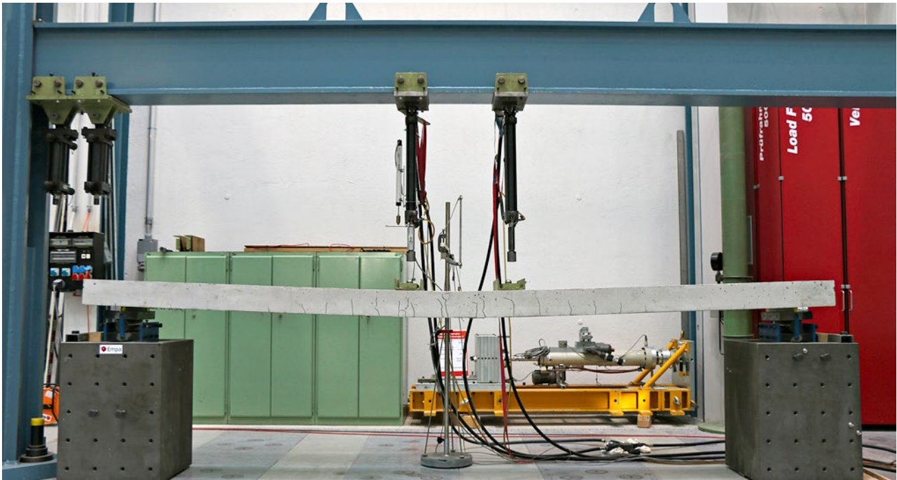
Concrete slab, test at Empa Switzerland
