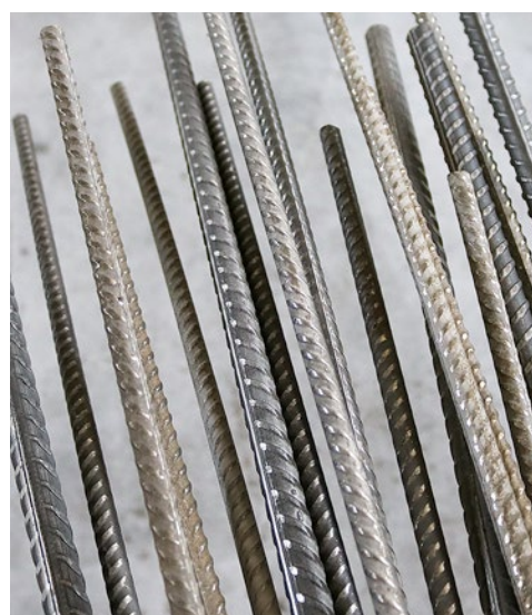
Ribbed bar similar to a 1.4003 alloy according to DIN EN 10088 (corrosion resistance class I)
